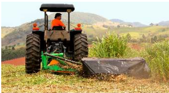
Driven by cardan shaft and belt transmission
