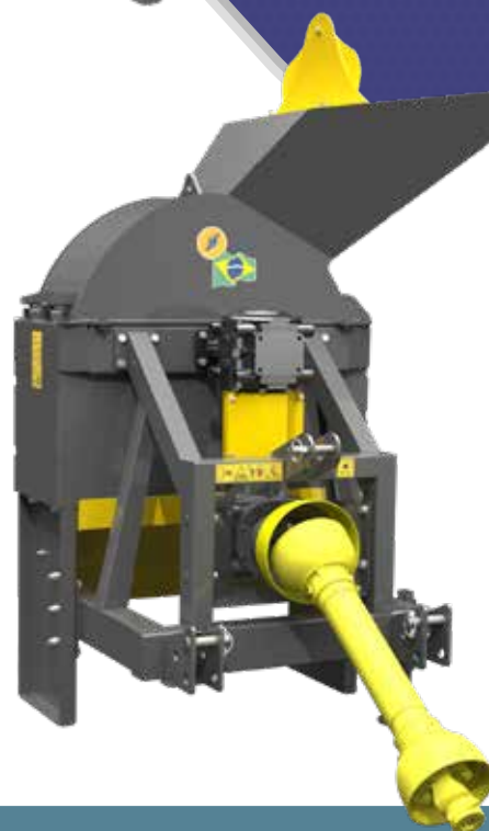
Driven by the tractor PTO
